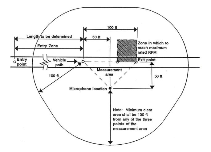
Figure 7.2-1. Test Site - Configured unidirectional for left to right acceleration from constant speed.
